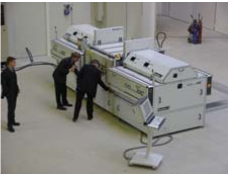
CVD Chemical Vapour Deposition Machine in the CONDIAS production plant ©pictures by hirseweb
